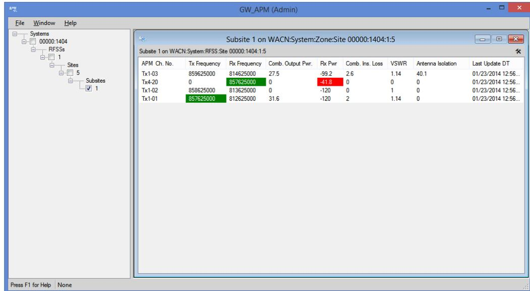
The screenshot shows the GW\_APM (Admin) interface. On the left is a tree view with 'Systems' expanded to '00000:1404', then 'RFSSs', '1', 'Sites', '5', and 'Subsites', with '1' selected. The main window displays 'Subsite 1 on WACN:System:Zone:Site 00000:1404:1:5'. Below this is a table with the following data:
