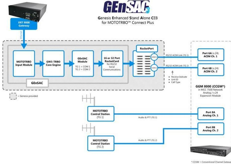
**Figure 1.1 – GW3-TRBO with GEnSAC Solution (Connect Plus)**
