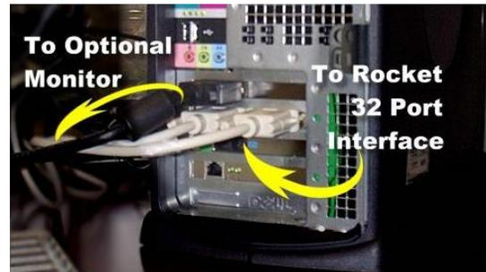
You may have purchased a 4-, 8-, 16- or 32-port GEnSAC. To keep things simple, we are supplying a RocketPort Card that is capable of up to 32 ports. If you have purchased a GEnSAC that is 16 or fewer ports, you will receive one port adapter “brick” (see below). If you order a GEnSAC capable of 32 ports, you will receive two port adapter “bricks” (see below). Depending on which version of the GEnSAC port interface you purchased, you will have received one of the following:
